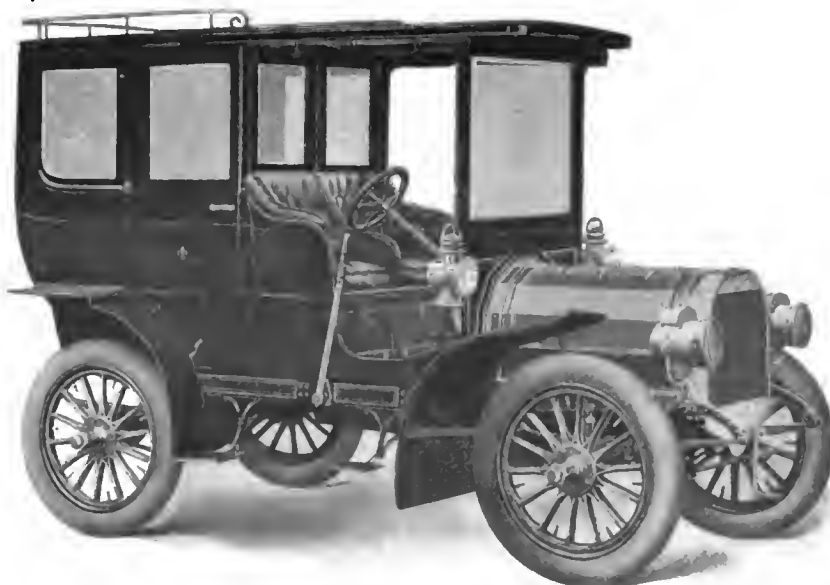
FIG. 1.—WELCH FOUR-CYLINDER CAR WITH SIDE ENTRANCE PULLMAN LIMOUSINE BODY.
